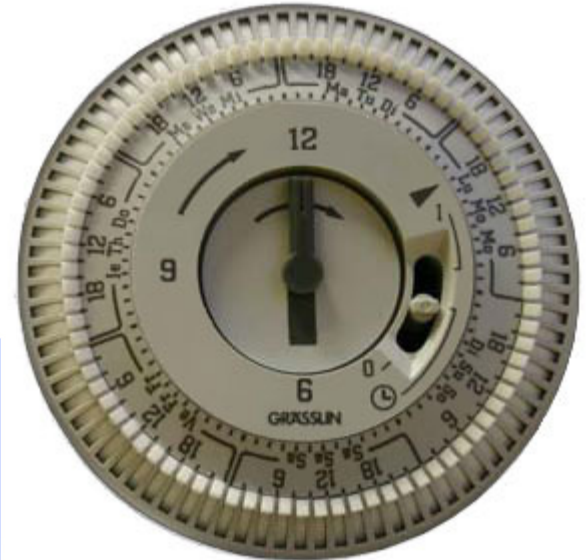
7-day timer dial: each tripper is 2 hours 24 hour dial: each tripper is 15 minutes
