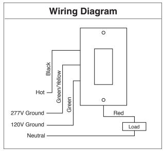
**NOTE**: 120VAC–Green wire can be connected to Neutral 277VAC–Green/Yellow wire can be connected to Neutral
