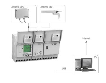
By external control input it is posible to switch selected channels permanently ON until next programmed command, to set countdown timer for selected channels, as well as to enable impulse counting.
