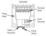
The TOWERCHRON QM1 and QM2 are both double insulated so earth protection is not required. However in the backplate a terminal for earth continuity is provided which should be used if earth conductors are present in your cable. Make sure that the earth conductors are sleeved to prevent accidental contact with live parts.
