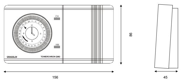
QM2 – two channel programmer. Independent control of heating and hot water
