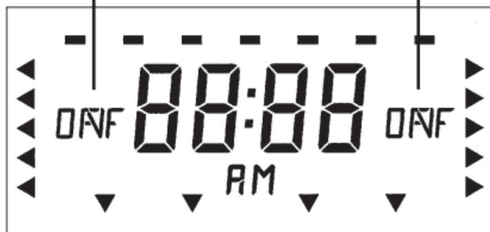
ON and OFF times for **HEATING** and **HOT WATER**
