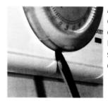
Align the bar on the edge of the cover with the groove at the lower edge of the dial in the housing. Remove the cover by applying a screw driver between groove and cover.
