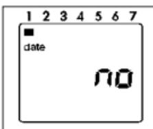
Press the + 1h as often as necessary until **no** appears. The time switch has no programmed date reference!
