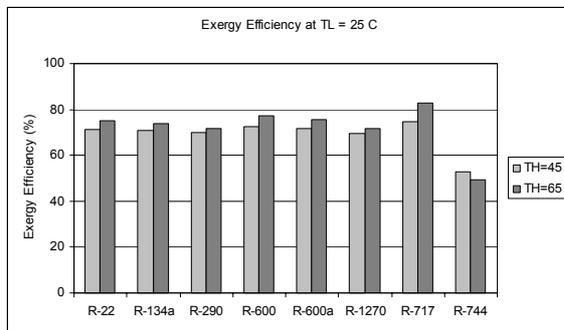
Fig. 11 Exergy efficiency of the heat pump system
