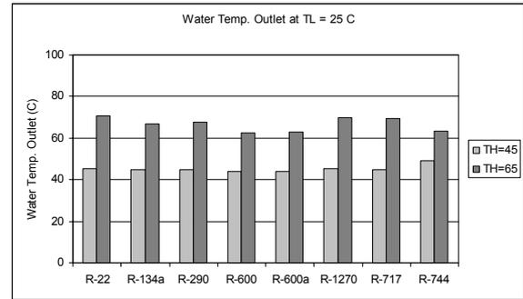
Fig. 7 Effectiveness of condenser and gas cooler in the heat pump system.
