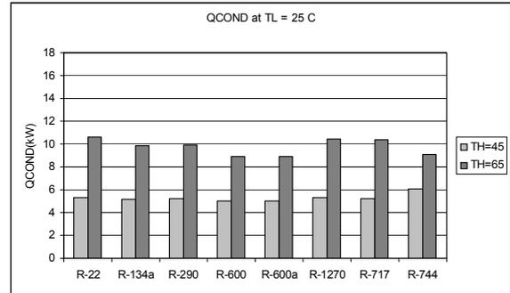
Fig. 6 Heat capacity at condenser / gas cooler of the heat pump systems.
