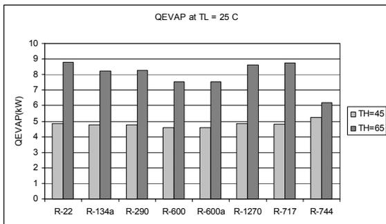
Fig 8 Heat capacity of evaporator in the heat pump system.
