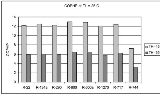
Fig. 10 Coefficient of performance of the heat pump system
