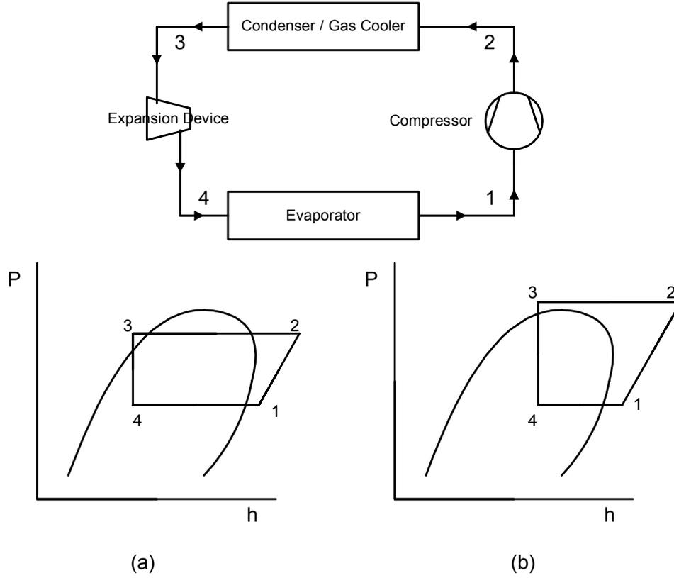
Fig. 1 P-h Chart for heat pump water heater system
