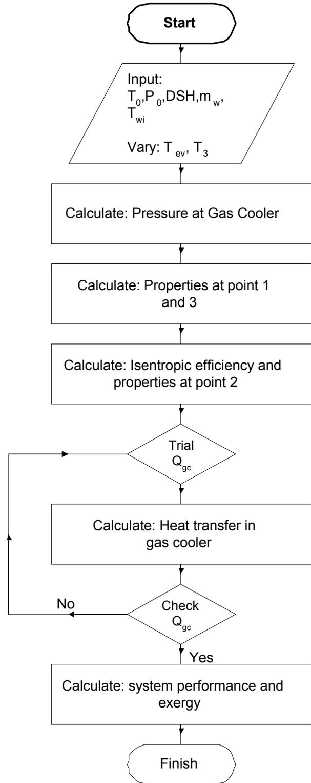
Fig. 2 Flow diagram of R-744 system
