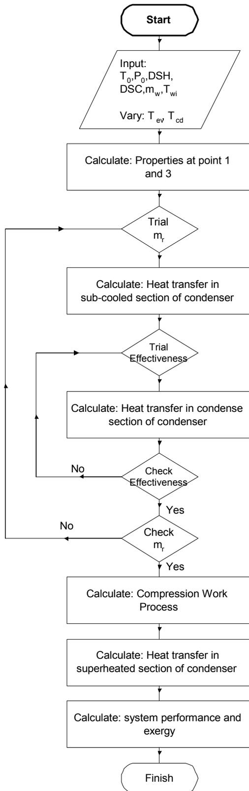
Fig 3 Flow diagram for working fluids except R-744
